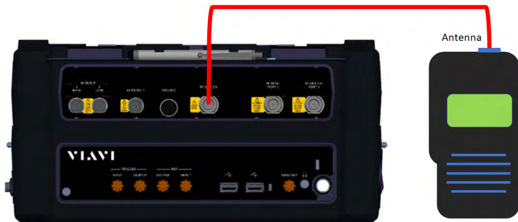
Figure 3-1 P25 Transceiver Test Setup Diagram
